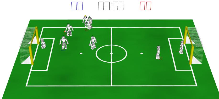
**Fig. 3.** A simulated game. The red and blue drawings on the field display the estimates of the current robot positions. The small dots above the robots show their current side confidence. Either a robot is certain to be in its own side (bright green, both goalies are certain), it is fairly sure about its playing direction (dark green), it is uncertain (yellow), or it is lost (red, not shown).
