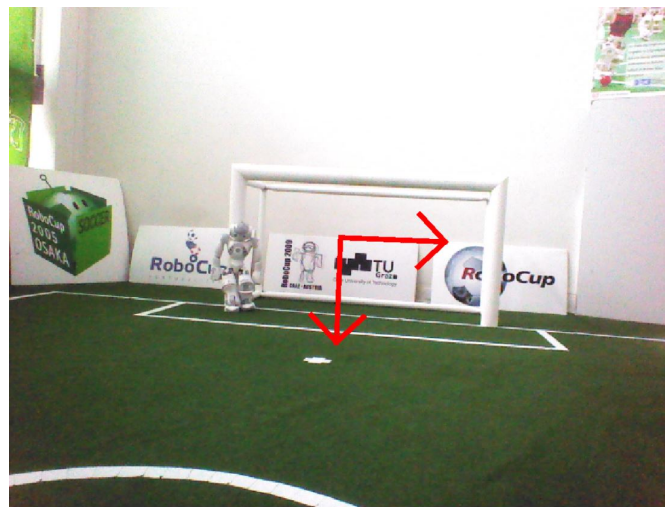
Figure 4.4: Origin of the ImageCoordinateSystem
