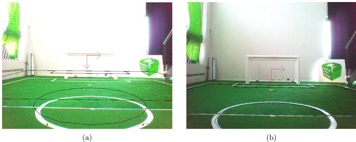
Figure 2.1: Projected lines before (a) and after (b) the calibration procedure
