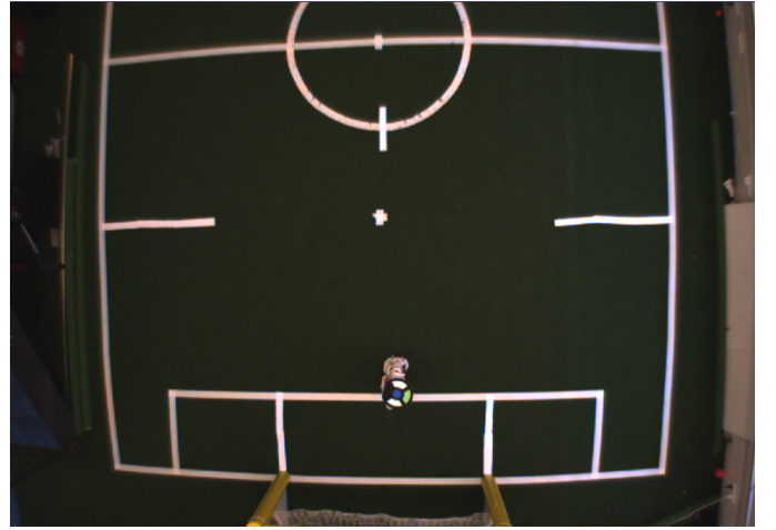
Fig. 9. Image taken by one of the cameras providing ground truth data. In the lower center, a tracking pattern on a robot's head can be seen. The field has intentionally a wrong line layout (cf. Tab. I, experiment 6).
